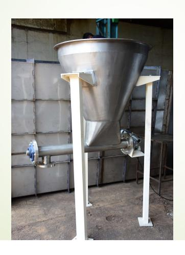
Application (Sand supply core making machine), Customer (Compax Industrial Equipments)
